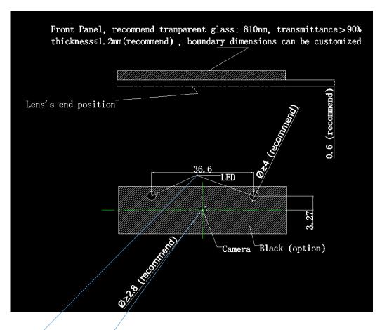
Fill-in light. Infrared light, 810nm, transmittance 85% or transparent;
